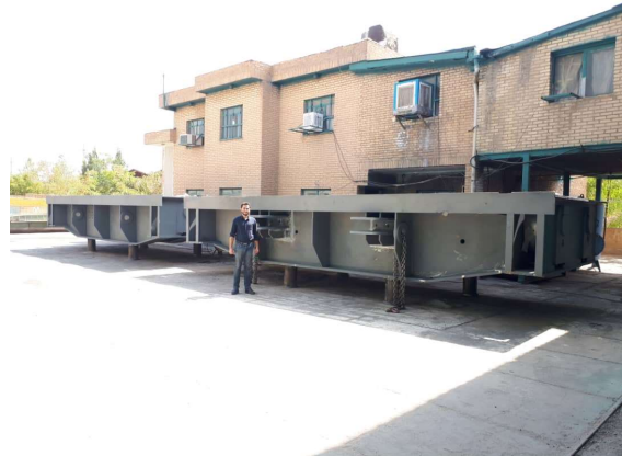
Khersan Dam Diversion Gate
