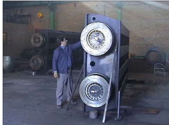
BOTTOM OUTLET GATE
