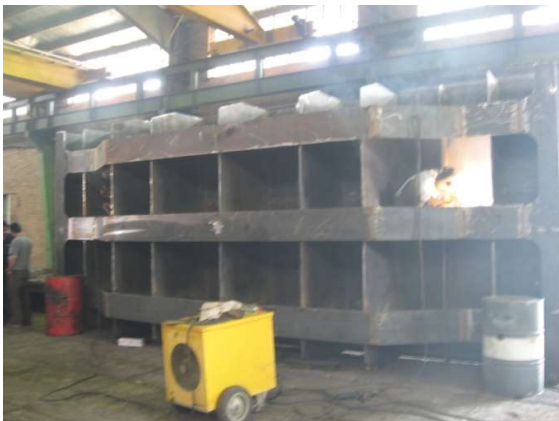
INTAKE STOPLOG MANUFACTURING
