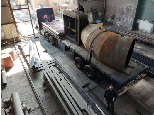
Transition and Bendpipe DN 2000
