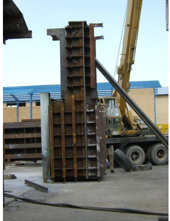
DRY TEST OF GATE & CASING
